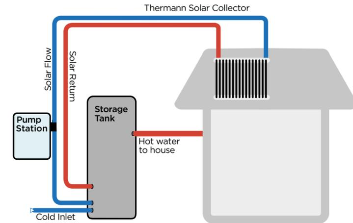
Note: Diagram not to scale - basic system overview (not installation guide).
